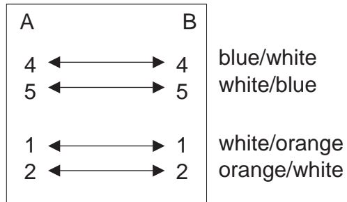
FIGURE 3-6. U-Net Cable Pairs and Pin-out
